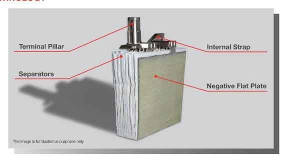
FIAMM FGL RANGE USE AGM (ABSORBED GLASS MAT) TECHNOLOGY. THE ELECTROLYTE IS ABSORBED IN FIBERGLASS SEPARATORS WITH 99% INTERNAL GAS RECOMBINATION EFFICIENCY. BLOCS ARE GRANTS NON-SPILLABLE AND MAINTENANCE FREE THEREFORE REQUIRES NO TOPPING UP OF ELECTROLYTE DURING ITS WHOLE LIFE. LOW SELF-DISCHARGE ALLOWS 6 MONTHS SHELF LIFE.
